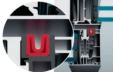
To open the window, the button is pressed again. The air escapes and the seal returns to its original, rolled-up position.
