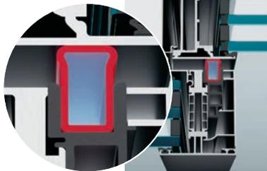
Pressing the button allows air into the frame. It is then pumped into the seal, causing the seal to press against the slider profile and completely seal the gap between the slider and the fixed frame.
