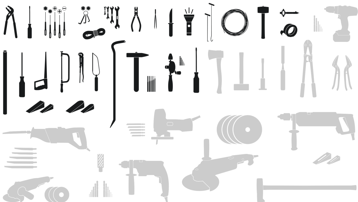
Selection of tools for RC1 to RC3 practical burglary testing
