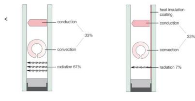
Energy transport insulating glass; without thermal coating
