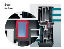
Pressing the button allows air into the frame. It is then pumped into the seal, causing the seal to press against the slider profile and completely seal the gap between the slider and the fixed frame.
