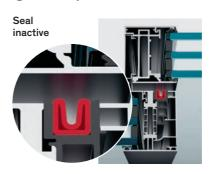
To open the window, the button is pressed again. The air escapes and the seal returns to its original, rolled-up position.
